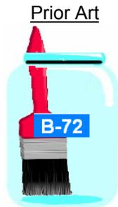
B-72 was known in the prior art, but only came in solid pellets that were mixed with a solvent by the user to form a liquid that was used only as a varnish, not as an adhesive. B-72 will quickly dry out when kept in a jar due to air exposure
